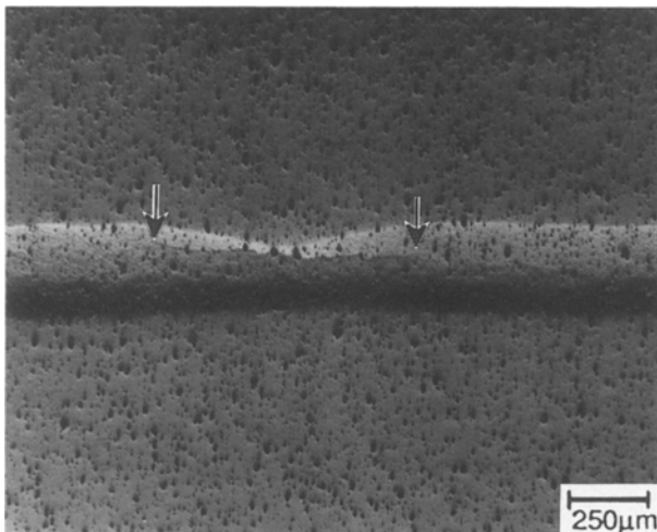
Figure 4 Surface crack within the primary transformation band in the three-point bend specimen of CeO 2 -TZP (Type IIA).
